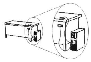
2. Insert the receiver's captive USB cable connector into an available USB receptacle on your computer.
