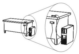
Insert the receiver's captive USB cable connector into an available USB receptacle on your computer.
