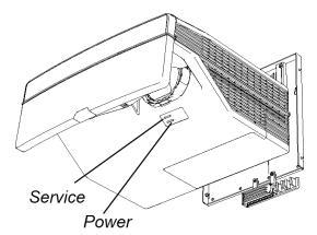
• The ECP's **Power** U button (see *Using the Extended Control Panel (ECP)* on page 15) also functions as a status light.
