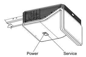
The ECP's Power (b) button (see Using the Extended Control Panel (ECP) on page 23) also functions as a status light.
