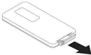
2. If you're accessing the remote control battery for the first time, remove the plastic sheet inside the battery holder, and then place the CR2025 coin cell battery in the battery holder.
