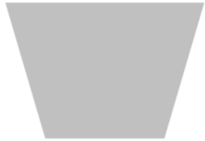
From the projector, the image path is too short along the bottom.
