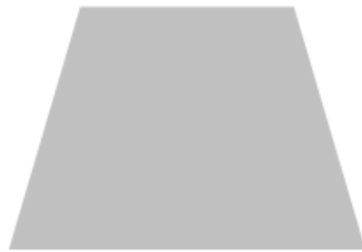
From the projector, the image path is too short along the top.
