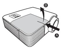
3. Remove and dispose of the lamp protection film.
