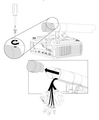
5. Loosen the locking screw and the knob on the projector mounting plate.
