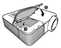
11. Replace the outer lamp cover, and then replace the screws holding the cover to the projector.
