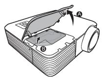
4. Using the screwdriver, loosen the screw on the lamp module.
