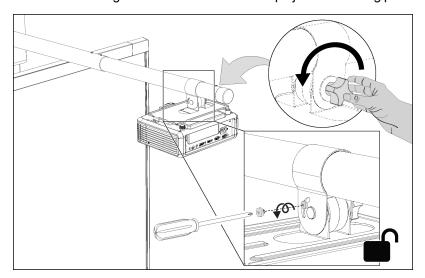
6. Slide the projector mounting plate and projector off of the boom.
