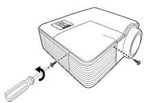
2. Remove the lamp cover, and then set it and the two screws aside in a safe place.
