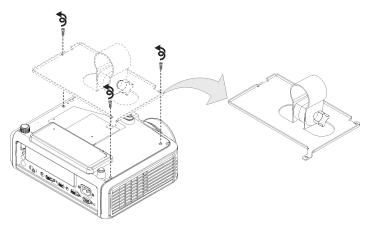
8. Turn over the projector so that the outer lamp cover is visible.
