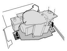
9. Using the screwdriver, tighten the screw on the lamp module.
