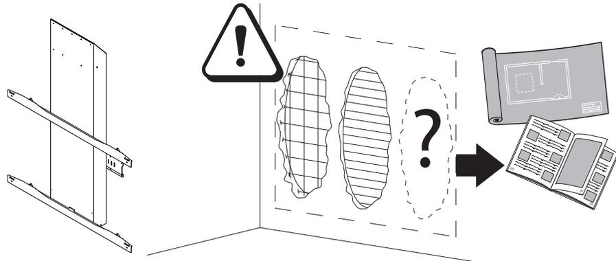
Your SMART product includes instructions and parts for installation on metal and wood stud walls and certain masonry wall types only. In the event that you need to install your SMART product on reinforced concrete walls, walls with plaster lath finishing, walls of unusual construction or other types of walls, refer to your local building authority for instructions, recommendations, and safe work practices.
