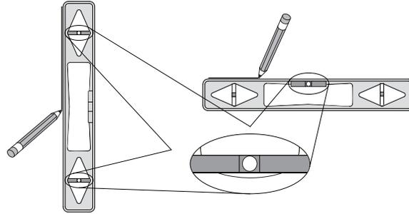
All of the lines that you draw to install the HAWM-UX/UF must be straight and level on a plumb wall. You must install the unit straight, level and plumb for it to operate properly.
