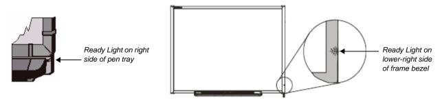
**3** Log on, if required, using the computer keyboard. When the Ready Light on the pen tray turns green, the computer and the interactive whiteboard have established communication. The board is now touch sensitive, and you can open any application available on the connected computer.
