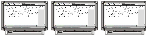
To set up multiple screens that display identical computer desktops, you'll need to either connect the projectors to each other in a daisy-chain pattern or install a video-distribution amplifier between the projectors and the computer.
