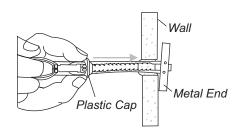
Slide the plastic cap to the drywall.
